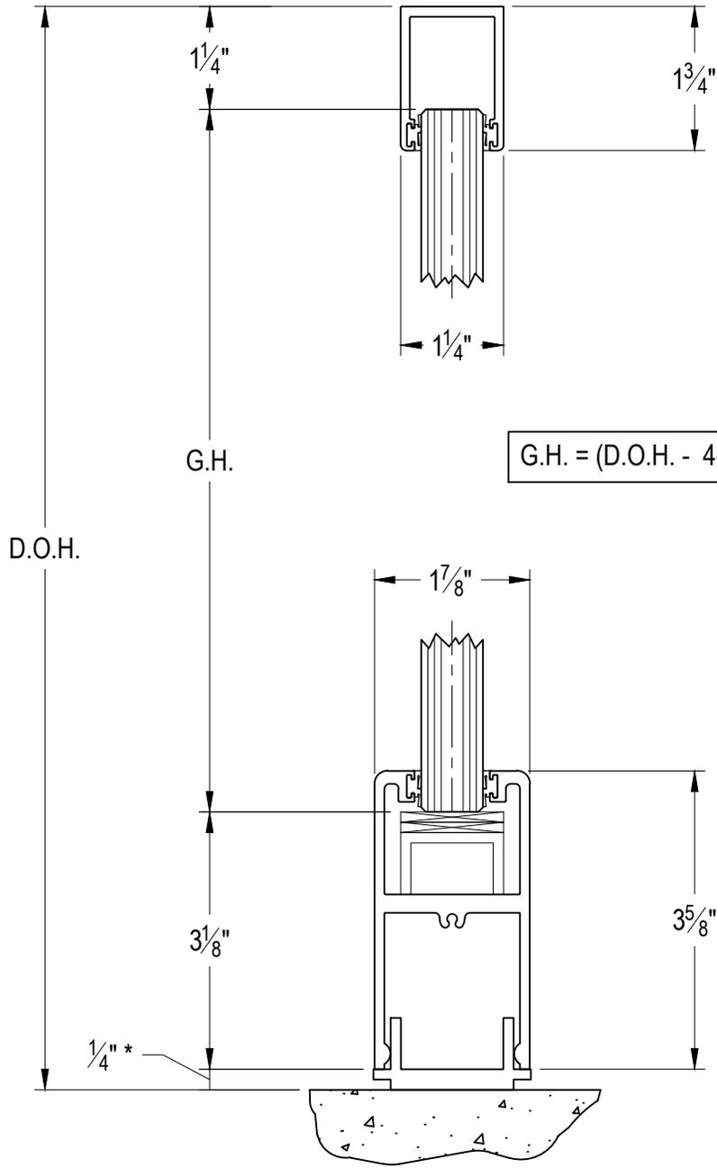
\* OPENING CLEARANCES MAY VARY BASED ON SITE CONDITIONS. STANDARD CLEARANCES SHOWN ARE USED IN FORMULA.
